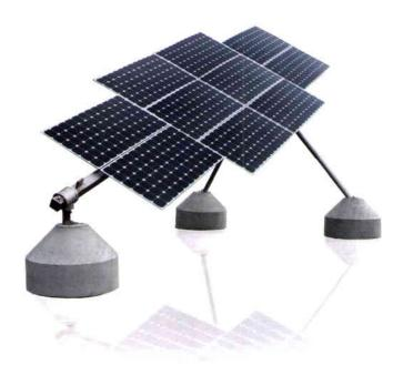
The SunPower T20 Tracker is the next generation in SunPower solar tracking technology. Built on the same proven, reliable design of the original PowerTracker®, the T20 Tracker represents the ideal combination of solar technology performance and system scalability. By tilting high-efficiency SunPower panels at 20-degrees and tracking on a single-axis to follow the path of the sun, the T20 Tracker generates up to 30% more energy than traditional fixed-tilt systems.
